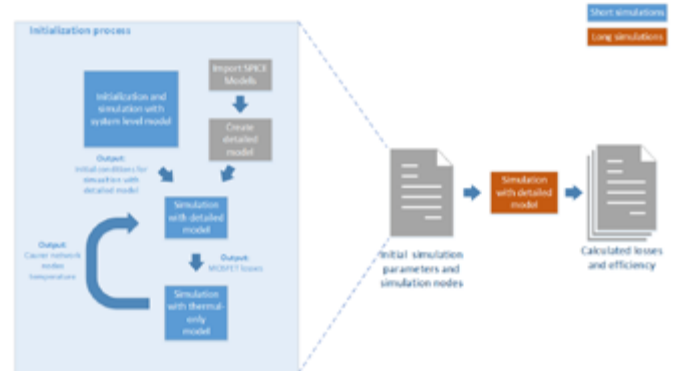
Figure 8: Proposed simulation flow for switching power converters
